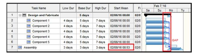
This effect is called Merge Bias. It occurs because duration of the fabrication of individual components is not completed at the same time. These durations are not correlated. For example, fabrication of Component 1 may take longer; but at the same time, fabrication of Component 2 may take shorter period if time. Start time of "Assembly" is calculated based on longer duration of activities "Component ...".
